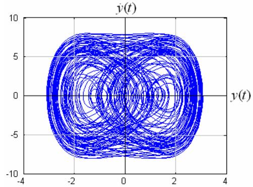
Fig 9. Phase path of chaotic Duffing system (1)
