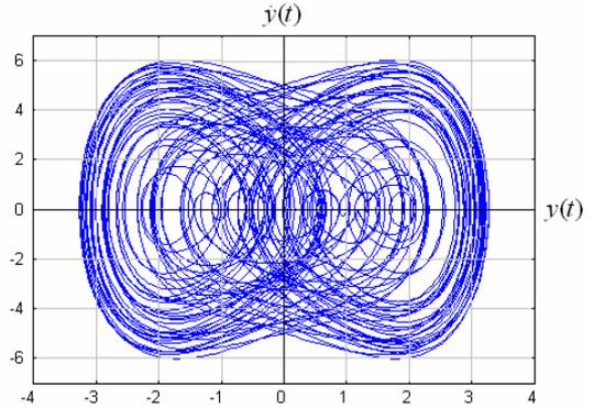
Fig 2. Phase path of chaotic Duffing system (1)
