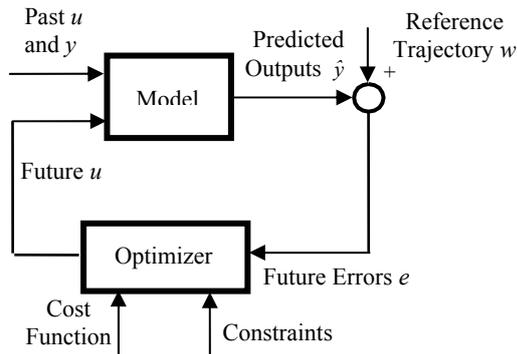
Figure 2. Block diagram of basic structure of MPC
