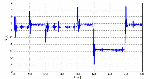
Figure 10. Control of DR300 using MPC STC (linear criterion).
