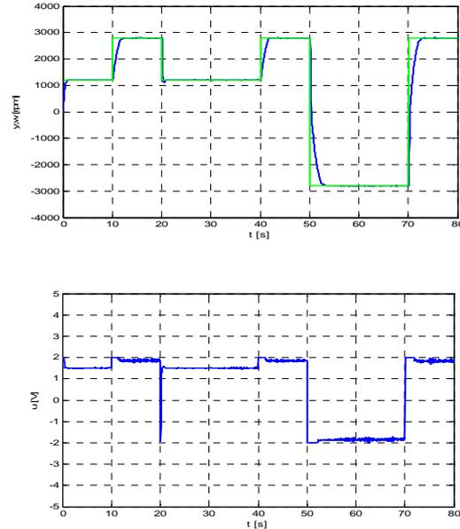
Figure 7. Control of DR300 using LQ STC (constrained case).
