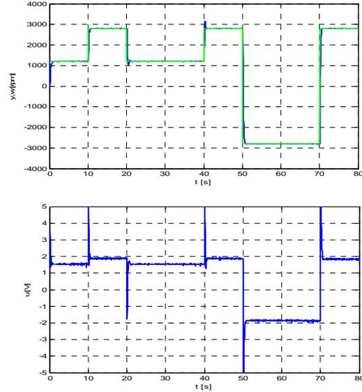
Figure 6. Control of DR300 using LQ STC (unconstrained case).
