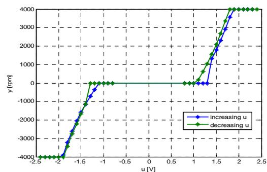
Figure 5. Static characteristics of Amira DR300 servomotor
