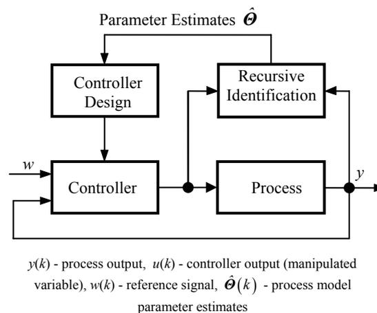
Figure 1. Block diagram of an explicit self-tuning controller
