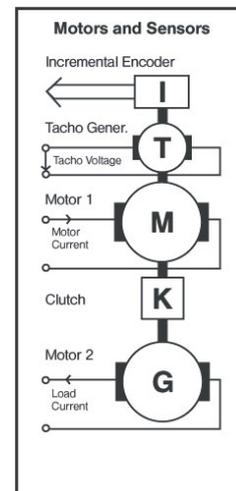
Figure 4. Block scheme of Amira DR300 servomotor.
