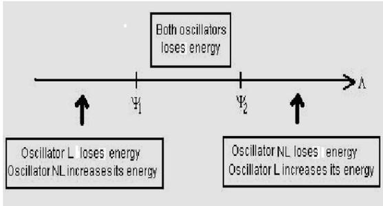
**Figure 1: Conditions for energy transfer between oscillators (L for linear and NL for nonlinear oscillator)**
