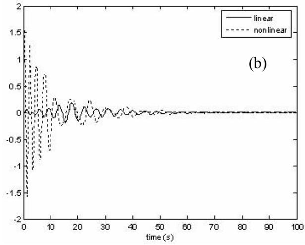
**Figure 3: Energy transfer from nonlinear to linear oscillator.
