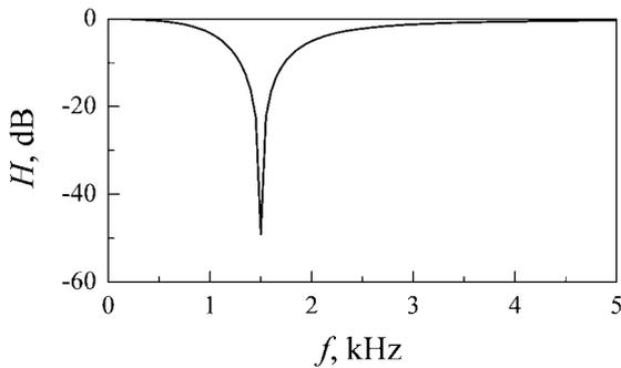
Figure 3. Transfer function  $H$  of the linear resonator.  $L_1 = 47$  mH,  $C_1 = 240$  nF,  $r = 1 \Omega$  ( $f_1 = 1.5$  kHz).
