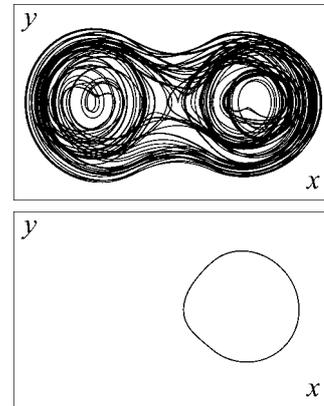
Figure 7. Phase portraits from Eq. (10). (top) without control,  $k = k_1 = 0$ , (bottom) under control,  $k = 1$ ,  $k_1 = 0.5$ . Other parameter values:  $a = 0.4$ ,  $b = 0.1$ ,  $b_1 = 0.01$ ,  $\Omega = \Omega_1 = 0.9$ .
