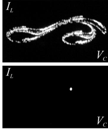
Figure 5. Stroboscopic maps (Poincaré sections). (top) without control, (bottom) under control. Parameters are in Fig. 3.
