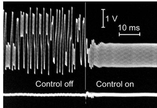
Figure 6. Experimental waveforms. Upper trace is the output signal  $V_C(t)$  and lower trace is the control signal taken across resistor R6. Fine vertical line in the photo divides the regions, where control is off and control is on. Parameters are in Fig. 3.
