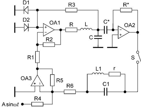
Figure 2. Circuit diagram of the two-well oscillator with the RNF controller in the feedback loop.  $\omega = 2\pi f$ . The S is an electronic switch.
