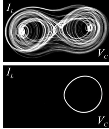
Figure 4. Phase portraits. (top) without control, (bottom) under control.  $A = 200$  mV,  $f_1 = f = 1.5$  kHz.
