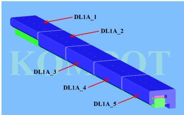
Figure 1. KOMPOT model of DL1A. Computed domain was reduced to one half of whole assembly due to symmetry.
