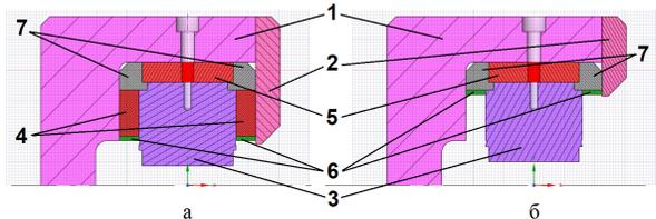
Figure 3. Components of modules DL1A2 to DL1A5 in 1/2 cross-section. 1 – iron yoke, 2 – side plate, 3 – pole, 4 – vertical PM, 5 – horizontal PM, 6 – Fe-Ni thermal shims, 7 – Al spacers.
