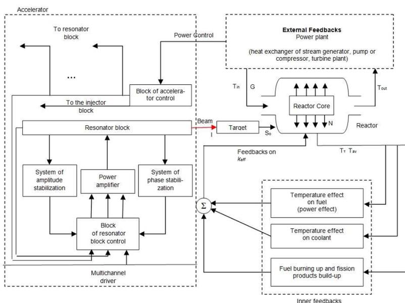
Figure 8. ADS structural scheme with feedbacks
