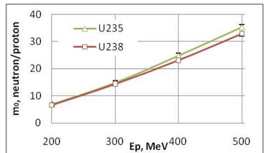
Figure 6. Neutron yields in the infinite uranic target (Geant 4.9.5).
