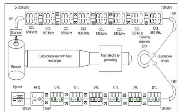
Figure 4. Possible ADS with proton linac scheme.
