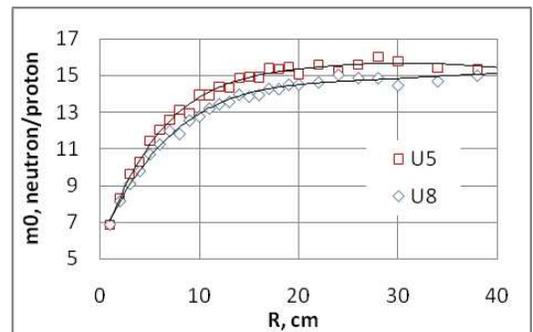
Figure 7. Dependence of spallation neutrons yield inside the target on its radius with 300 MeV proton beam (Geant 4.9.5).
