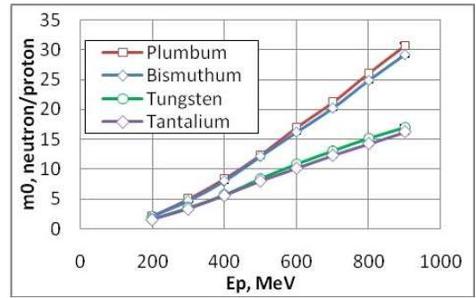
Figure 5. Neutron yield from target with the optimal sizes
