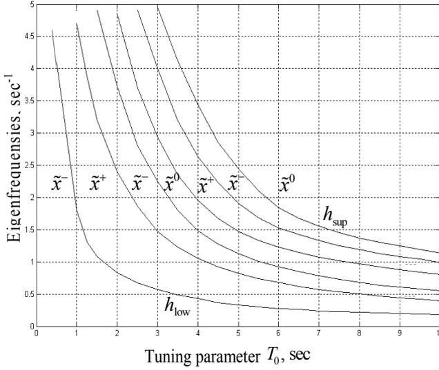
Fig. 1. Stability regions at the coefficient  $k_\omega = 0$ .
