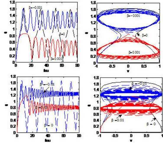
Figure 2. Plots of  $a(\tau)$  and phase portraits of system (6) with  $f = 0.2799$  and  $\beta = \pm 0.001$  (top row);  $f = 0.3412$  and  $\beta = \pm 0.01$  (bottom row). Plots of the LPTs corresponding to  $\beta = 0$  are shown for comparison.
