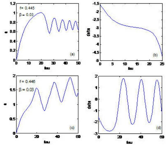
Figure 4. Plots of  $a(\tau)$  and  $\Delta(\tau)$  in tunneling ( $f = 0.445$ ,  $\beta = 0.03$ ) and autoresonance ( $f = 0.446$ ,  $\beta = 0.03$ ).
