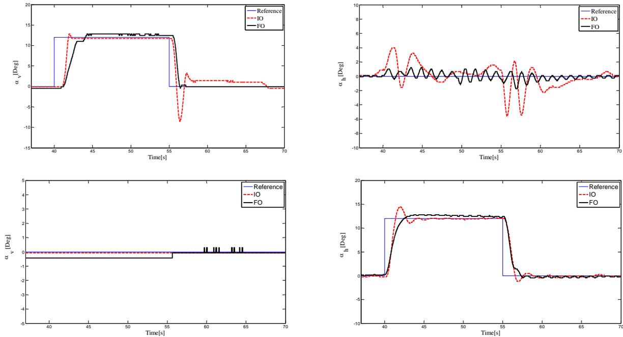
Figure 9 – Time responses of the experimental 2–dof helicopter for  $\alpha_v$  and  $\alpha_h$  using the  $PID$  and  $PID^\alpha$  controllers, for a pulse perturbation at the  $\alpha_{hr} = 12^\circ$  and  $\alpha_{vr} = 12^\circ$  position reference for sampling time  $h = 0.01$  s.
