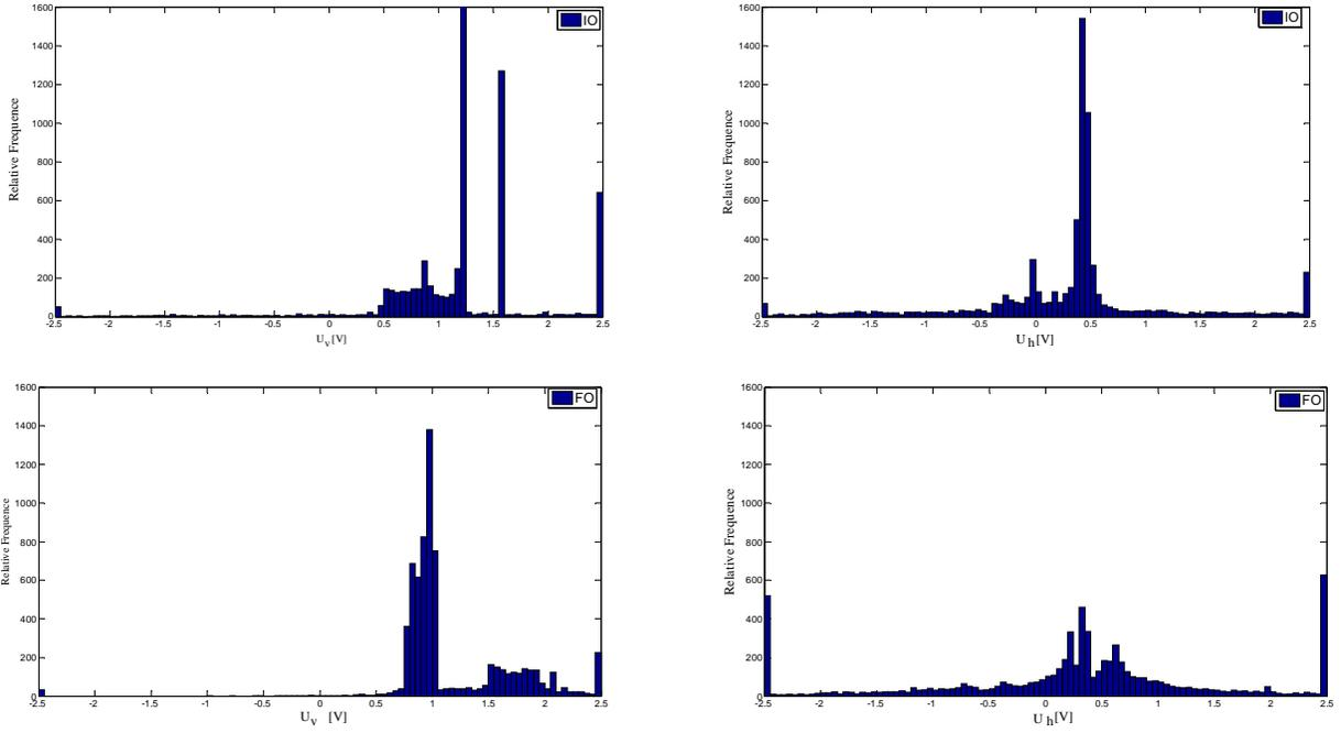
Figure 10 – The experimental 2-*dof* helicopter rotor and tail voltage statistical distribution using the *PID* vs *PID*<sup>α</sup> controllers, for a pulse perturbation  $\delta\alpha_v = 12^\circ$  at the  $\alpha_{vr}$  position reference for sampling time  $h = 0.01$  s.
