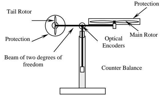
Figure 2 – The twin rotor mimo system.
