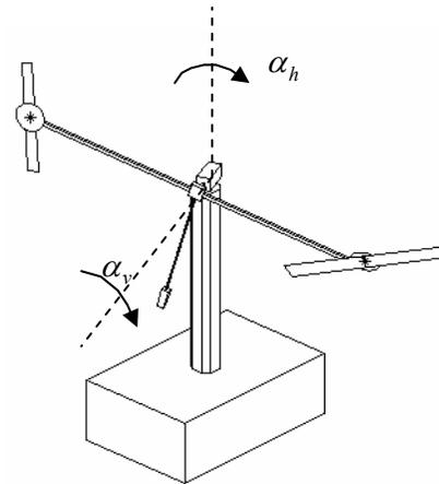
Figure 3 – The rotation of the helicopter system.
