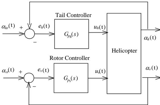
Figure 8 –Twin Rotor MIMO block PID control diagram
