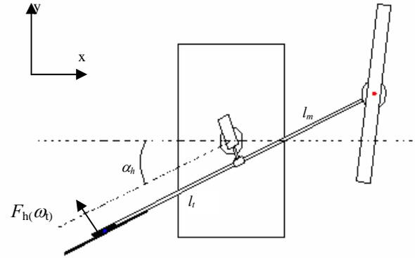
Figure 6 – Moments of forces in horizontal plane.
