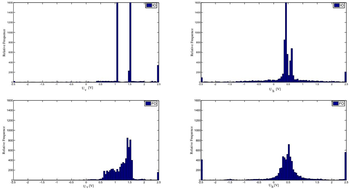
Figure 11 – The experimental 2-*dof* helicopter rotor and tail voltage statistical distribution using the *PID*<sup>α</sup> controllers, for a pulse perturbation  $\delta\alpha_h = 12^\circ$  at the  $\alpha_{hr}$  position reference for sampling time  $h = 0.01$  s.
