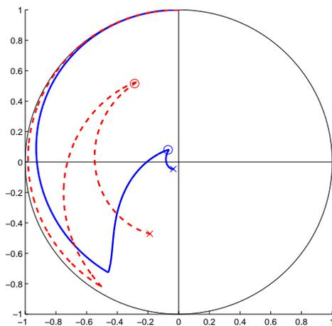
Figure 8. The state trajectory of the bang-exceptional arc of the non-saturation problem with  $t_1 = 0.4142$ . The spin  $q_1$  is shown as a solid blue line, with  $q_2$  as a dashed red line. The circle marks the point of highest contrast at  $T = 5.5734$ . For reference, the trajectory is continued past  $T$  until  $t_c = 7.3565$  when the first conjugate point, marked with an  $\times$  occurs.
