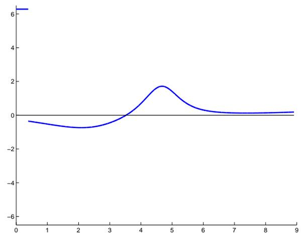
Figure 4. The control associated with the bang-exceptional arc of the saturation problem with  $t_1 = 0.3858$ .
