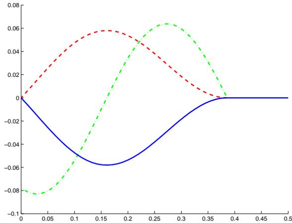
Figure 5. Components of the Hamiltonian for the bang-exceptional arc of the saturation problem with  $t_1 = 0.3858$ . The components are  $H_{F_0}$  in a dashed red line,  $uH_{F_1}$  in a solid blue line, and  $\{H_{F_0}, H_{F_1}\}$  in a dot-dashed green line. All three of these are identically zero on the exceptional arc, after the switching time  $t_1$ .
