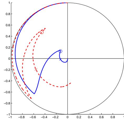
Figure 3. The state trajectory of the bang-exceptional arc of the saturation problem with  $t_1 = 0.3858$ . The spin  $q_1$  is shown as a solid blue line, with  $q_2$  as a dashed red line. The circle marks the point of highest contrast at  $t = 4.0376$ , which notably is not at the final time  $T = 8.9081$ . The conjugate point is marked with an  $\times$ .
