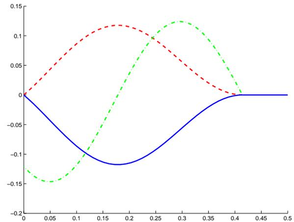
Figure 10. Components of the Hamiltonian for the bang-exceptional arc with  $t_1 = 0.4142$ . The components are  $H_{F_0}$  in a dashed red line,  $uH_{F_1}$  in a solid blue line, and  $\{H_{F_0}, H_{F_1}\}$  in a dot-dashed green line. All three of these are identically zero on the exceptional arc, after the switching time  $t_1$ .
