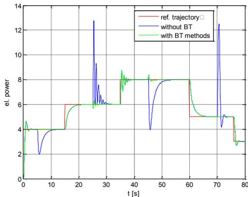
Fig. 13 Time responses of the electric power and reference trajectory (with and without BT methods)
