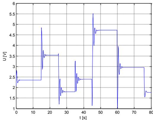
Fig. 10 Time responses of the controlled variable (with BT), respective to scheme 1
