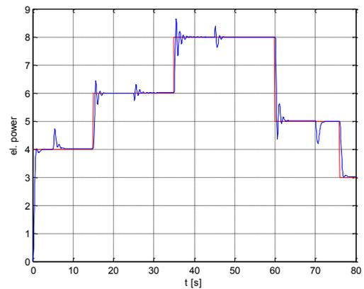
Fig. 7 Time responses of the electric power and reference trajectory
