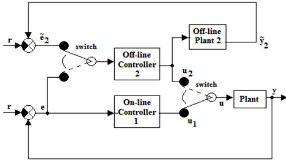
Fig. 2 Bumpless transfer scheme 2 for switching system dynamics
