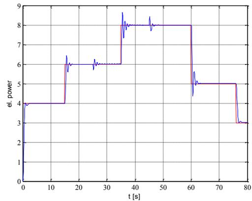
Fig. 11 Time responses of the electric power and reference trajectory (using both approaches: scheme 1 and 2)
