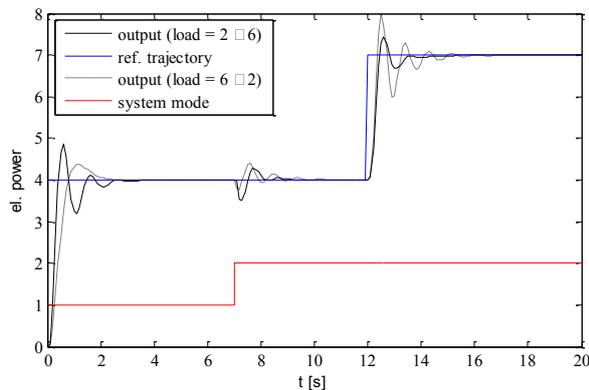
Fig. 5 Time responses of the system output during switching, load change from 2 to 6 (solid line), load change from 6 to 2 (dotted line)
