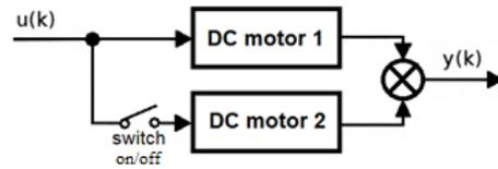
Fig. 3 Scheme of switched DC motors
