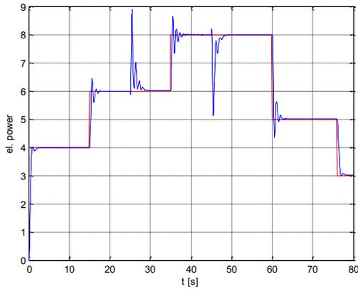
Fig. 9 Time responses of the electric power and reference trajectory (with BT), respective to scheme 1
