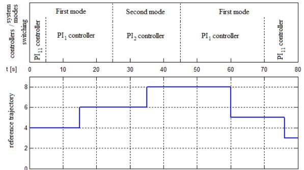
Fig. 6 Graphical illustration of system modes, controllers switching and the reference trajectory
