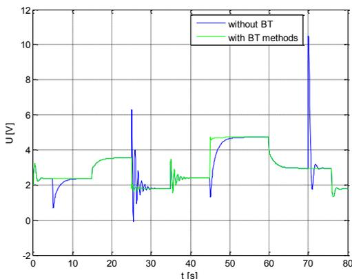
Fig. 14 Time responses of the controlled variable (with and without BT methods)
