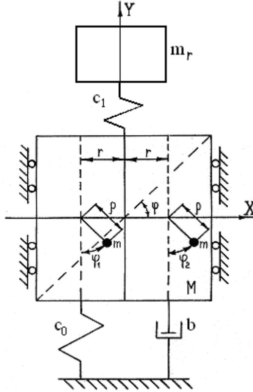
Fig.1. Scheme of the two-rotor vibration set-up.
