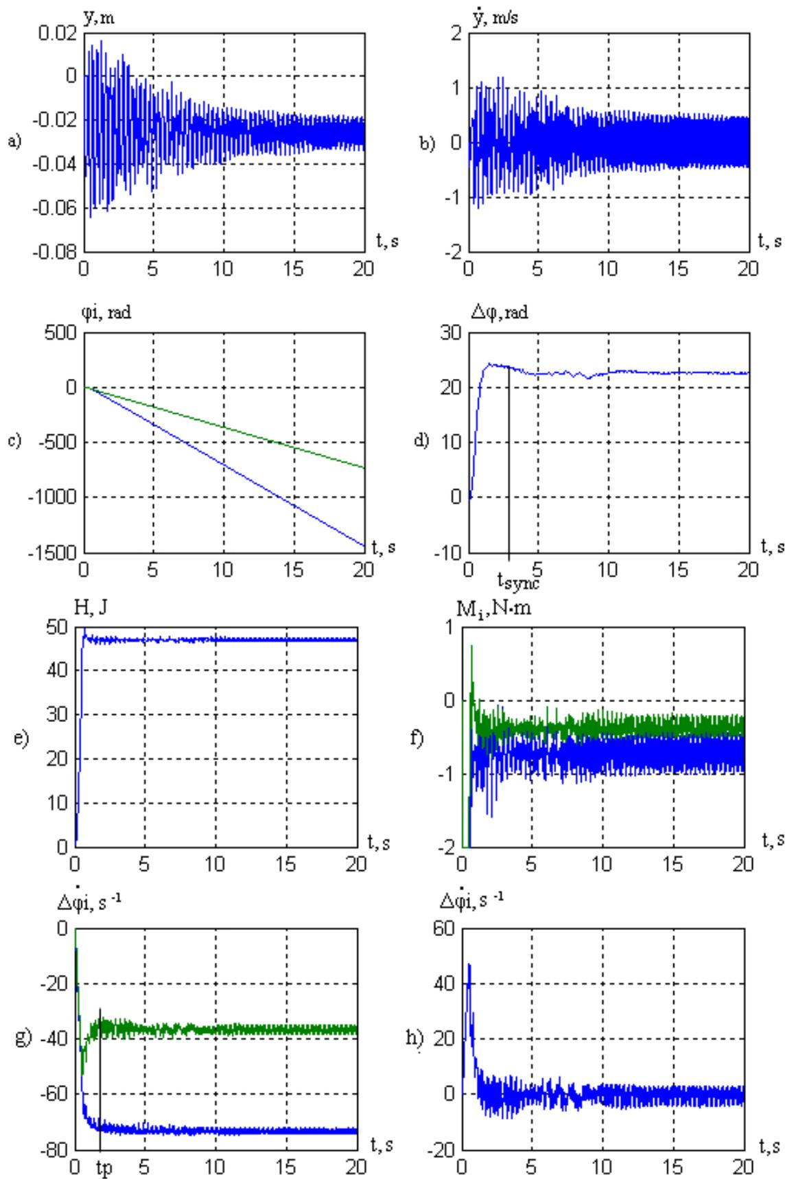
Fig.3. Simulation results for a system with bounded controlling torques,  $M_1 < 2 N\cdot m$ ;  $M_2 < 2 N\cdot m$ ,  $V = 1/3 kg/m$ ;  $t_2 = 8s$ .
