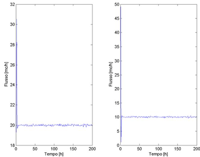
Figure 5. Simulation of LQG control of head and bottom product flow rates
