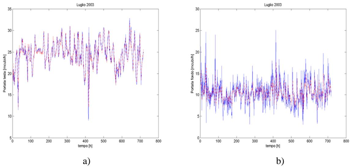
Figure 3: Fitting of head and bottom products flow rate
