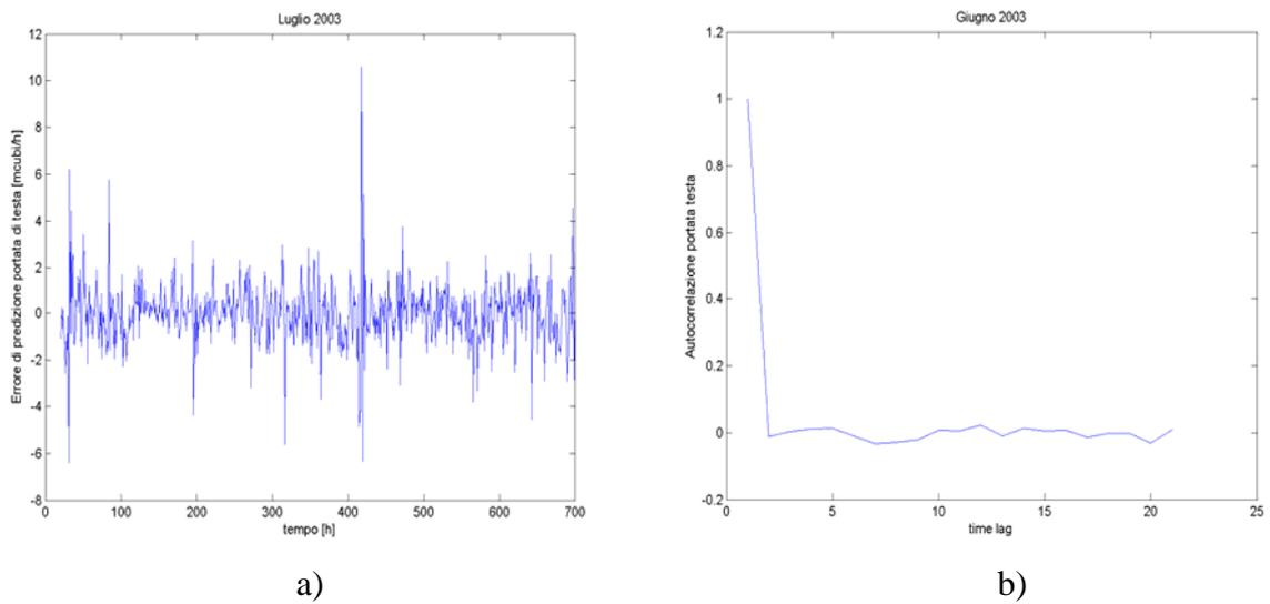
Figure 4: Prediction error for head product flow rate and relative autocorrelation function.
