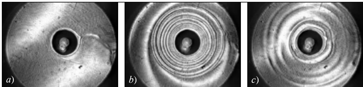
Figure 1. Interferograms of concentration field around the air bubble in horizontal layer of stratified isopropyl alcohol solution. t : 0 ( a ), 2.0 ( b ), 10.0 ( c ) sec.
