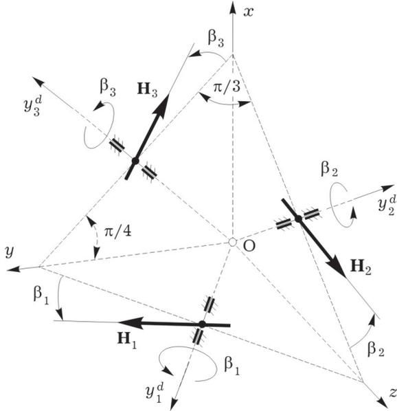
Figure 3. The GMC scheme *Star* by 3 gyroscopes
