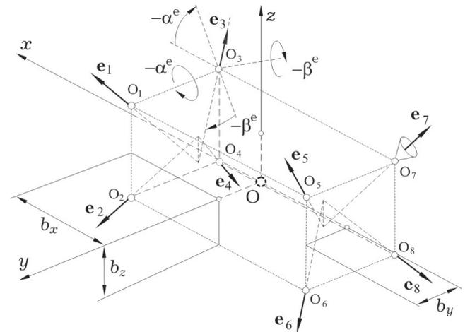
Figure 4. The CEU scheme by 8 electro-reaction engines
