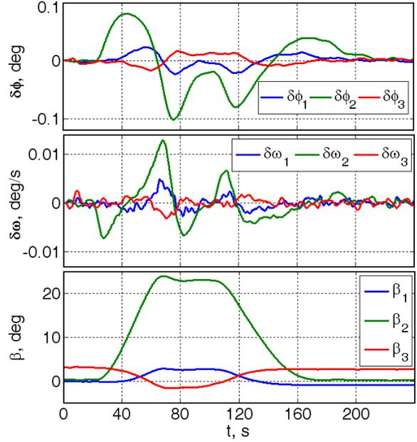
Figure 10. The SC attitude errors and the GD's angles
