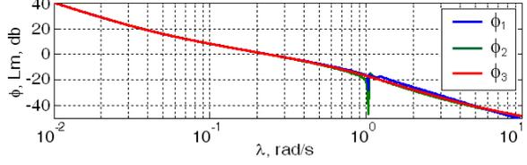
Figure 6. The discrete LAFC of the SC open-loop channels
