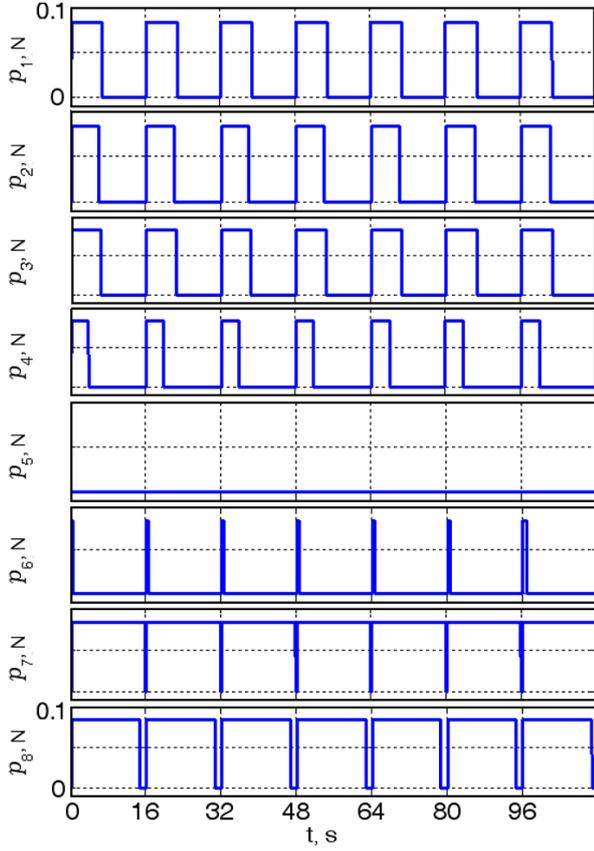
Figure 11. The time diagrams of current the ERE thrusts and the CEU normed pulses of force and torque
