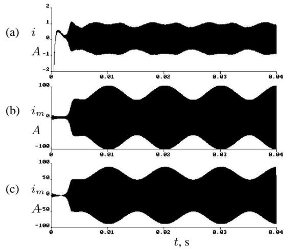
Figure 3. Simulation of the closed loop system for nonlinear magnetostrictive vibrator when modulated by a low frequency ((a) is an electric current  $\hat{i}$ ; (b) is an equivalent of the mechanical shift  $\hat{i}_m$ ; (c) is the same when doubled mechanical load).
