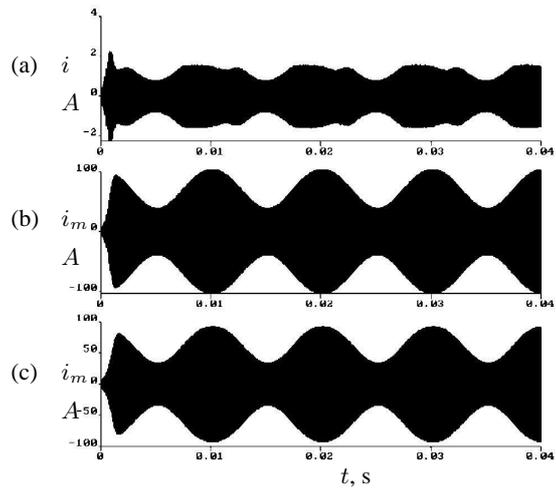
Figure 1. Simulation results for the closed loop system when modulated by a low frequency ((a) is an electric current  $\hat{i}$ ; (b) is an equivalent of the mechanical shift  $\hat{i}_m$ ; (c) is the same when doubled mechanical load).
