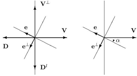
Fig. 1. Drag and lift forces and the angle of attack
