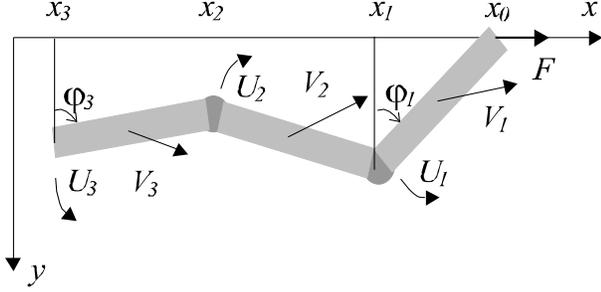
Fig. 3. The mechanical system of sequentially joined bodies
