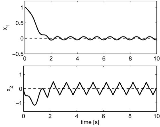
Figure 1. Responses of the perturbed double integrator (19) using the twisting algorithm with PD terms (20) and considering a sinusoidal perturbation.
