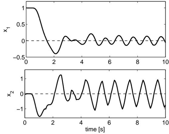
Figure 2. Responses of the perturbed double integrator (19) using the twisting algorithm (34) and considering a sinusoidal perturbation.
