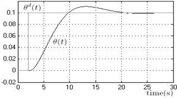
Fig. 3. Plots of the aircraft pitch attitude  $\theta(t)$  (rad) and  $\theta^d(t)$  (rad).
