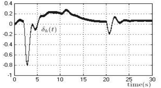
Fig. 8. Plot of the elevator deflection  $\delta_h(t)$  (rad).
