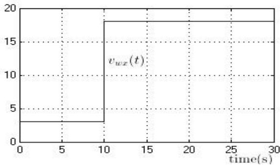
Fig. 11. Plot of wind gusts  $v_{wx}(t)$  (m/s).
