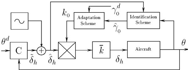
Fig. 2. Block diagram of the aircraft pitch attitude control system with adaptive gain tuning
