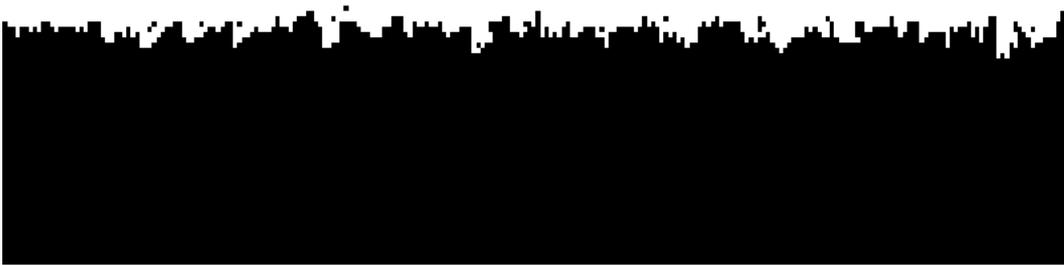
Figure 2: Random Etching (or Random Aggregation) Model: Uncorrelated stochastic etching, resulting in surface roughening. Underetching is possible, but occurs rarely.
