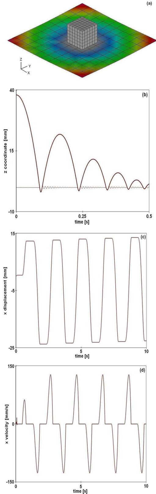
Figure 3. Elastic block hitting a thin flexible plate: (a) deformed geometry; (b) vertical displacement of a node on the lowest surface of the block (thick line) and vertical displacement of a nearby point of the plate (thin line); (c) horizontal displacement and (d) velocity of the same node of the block.
