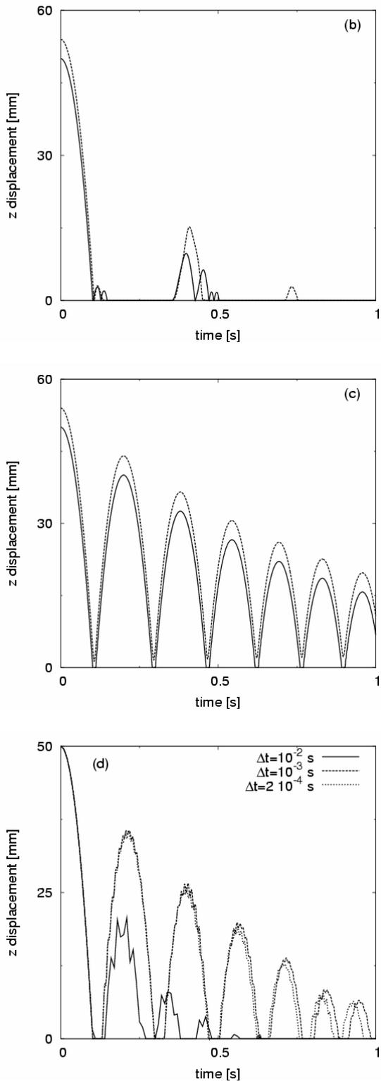
Figure 1. Elastic shell bouncing on rigid ground: (a) deformed geometry; (b) vertical displacement of a rubber shell; (c) vertical displacement of a steel shell and (d) effect of time step size on convergence.
