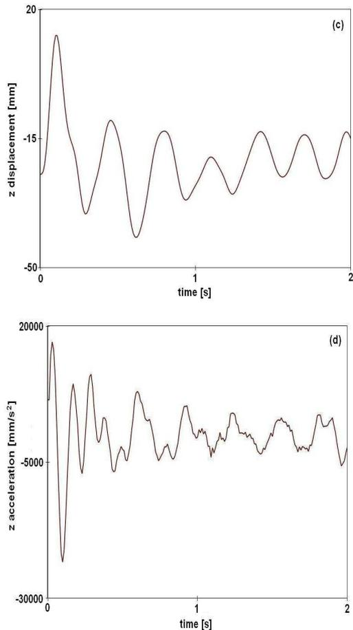
Figure 2. Prototype vehicle structure: (a) deformed geometry; (b) vertical displacement of the front left wheel (thin line) and road profile (thick line); (c) vertical displacement history and (d) vertical acceleration history, at point A on the frame of the vehicle.
