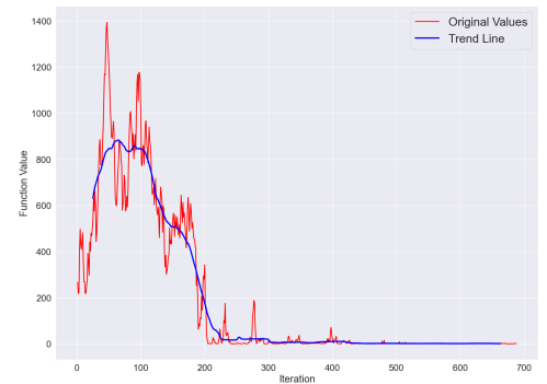
Figure 9: Red line: Sample path of the classical Simulated Annealing algorithm for Multiple Global Minima function. Blue line: fitted trend line.
