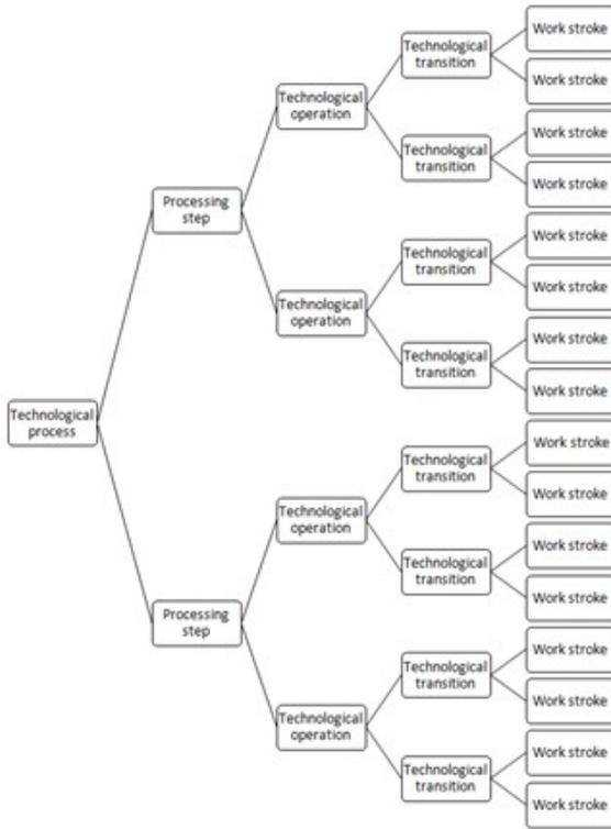
Figure 1. Structural model of the technological process of manufacturing the product on metal-cutting machines
