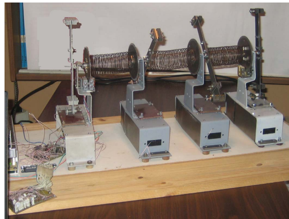
Figure 2. Photo of four coupled pendulum sections.
