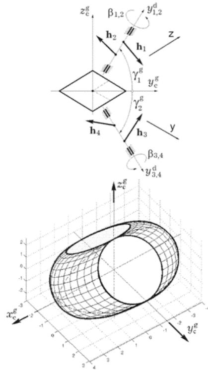
Figure 3. *2-SPE* scheme and envelope of its AM variation domain
