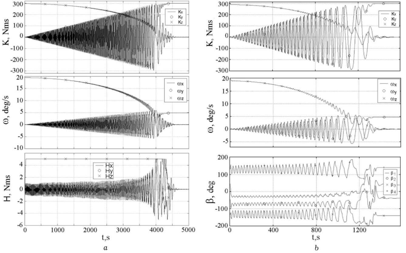
Figure 4. Dynamics of the RB respinup: *a* — by 3 reaction wheels; *b* — by 4 GDs on scheme 2-*SPE*.
