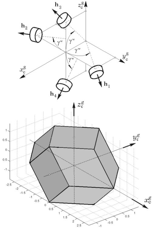
Figure 2. *GE* scheme and envelope of its AM variation domain
