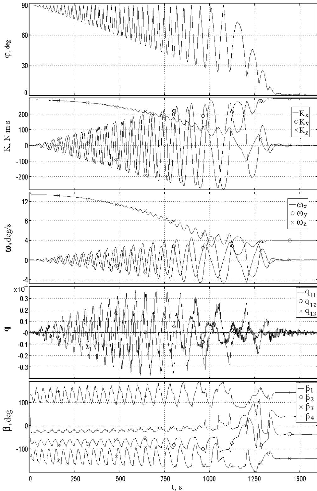
Figure 5. Dynamics of the flexible SC respinup by 4 GDs with own AM  $h_g = 7.5$  Nms and constrain  $u^m = 10$  deg/s
