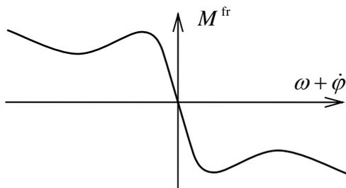
Figure 2. Friction moment function.
