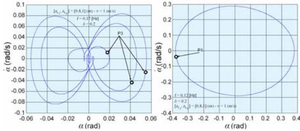
Figure 6 - Comparison of Poincaré maps between a periodic-3 orbit and the uncontrolled orbit
