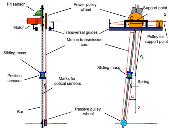
Sketch of a physical pendulum with moving mass and perturbed pivot
