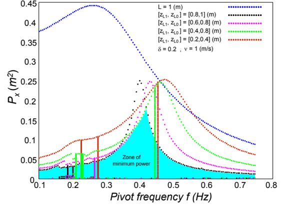
Figure 3 - Zone of minimum energy according to bifurcation diagrams with variable range of mass displacement
