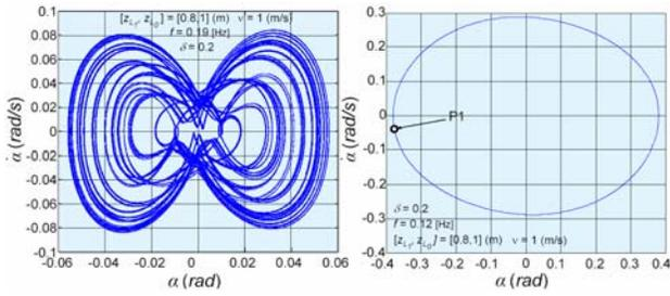
Figure 5 - Comparison of Poincaré maps between a chaotic orbit (strange attractor) and the uncontrolled orbit
