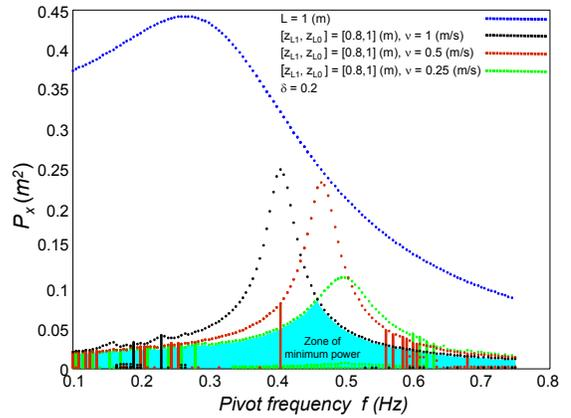
Figure 4 - Zone of minimum energy according to bifurcation diagrams with variable mass velocity
