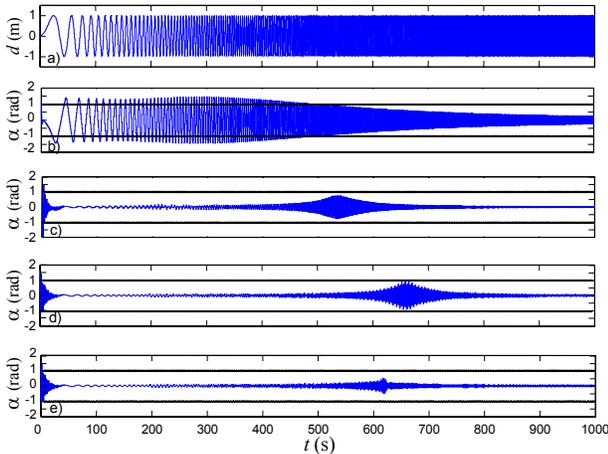
Figure 8 - a) Pivot motion in chirp form with  $f$  from 0 (Hz) up to 0.75 (Hz). b) without controller. c) Low-frequency controller. d) High-frequency controller. e) Knowledge-based switching controller.
