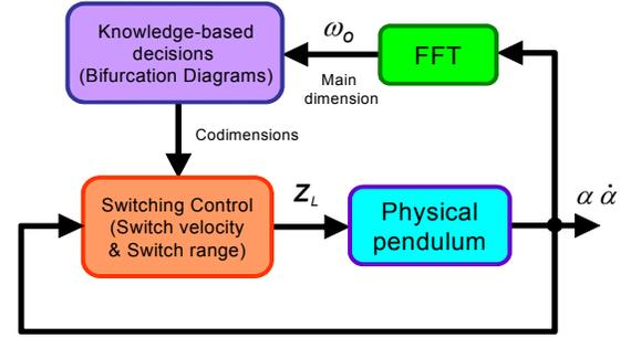
Figure 7 - Knowledge-based control diagram
