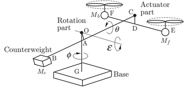
Fig. 1. Overview of a model helicopter.
