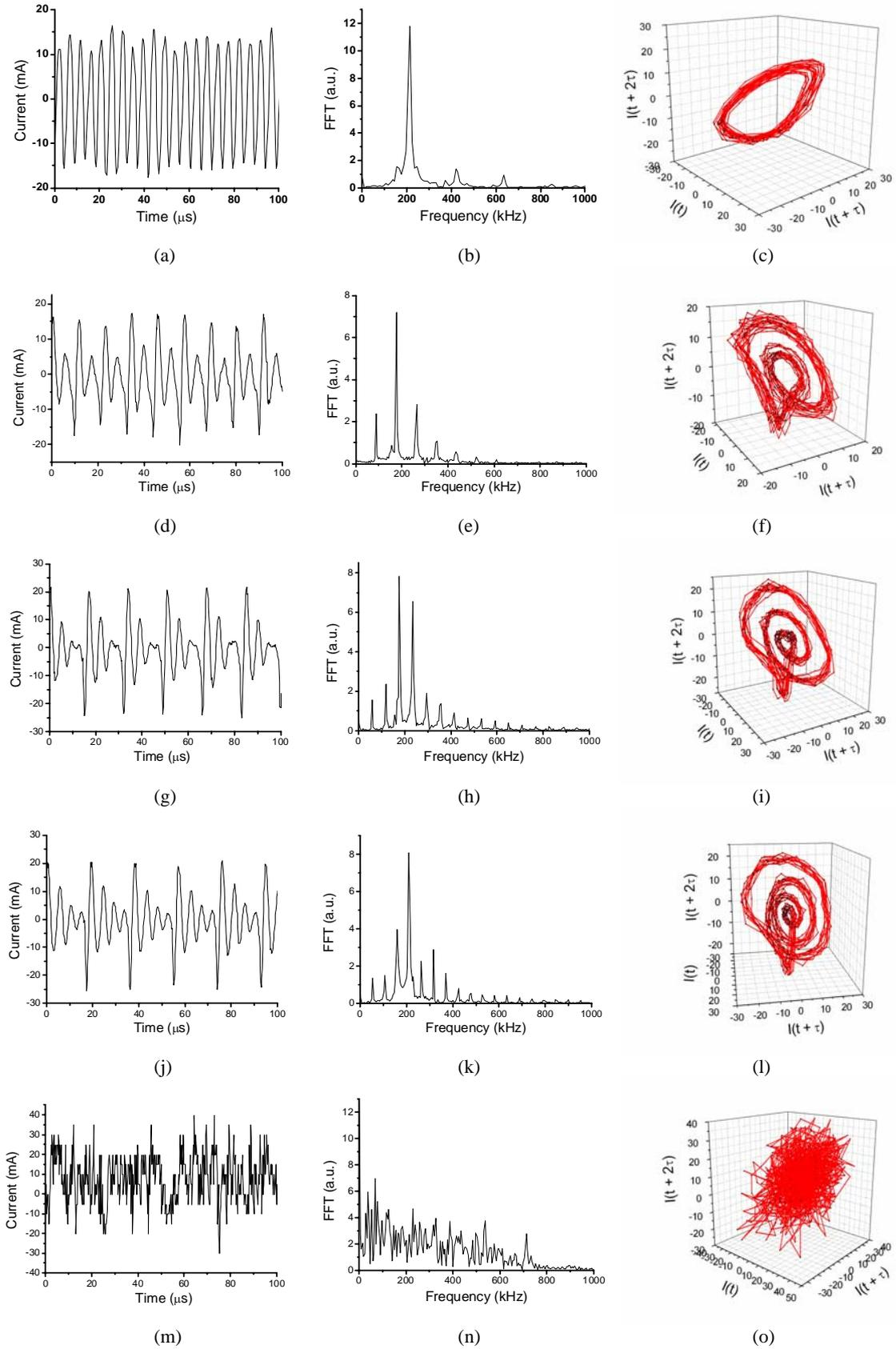
Fig. 2: Oscillations of the current (first column), their FFT's (second column) and the reconstructed attractor of the plasma system dynamics (third column), at different increasing values of the potential applied on the electrode
