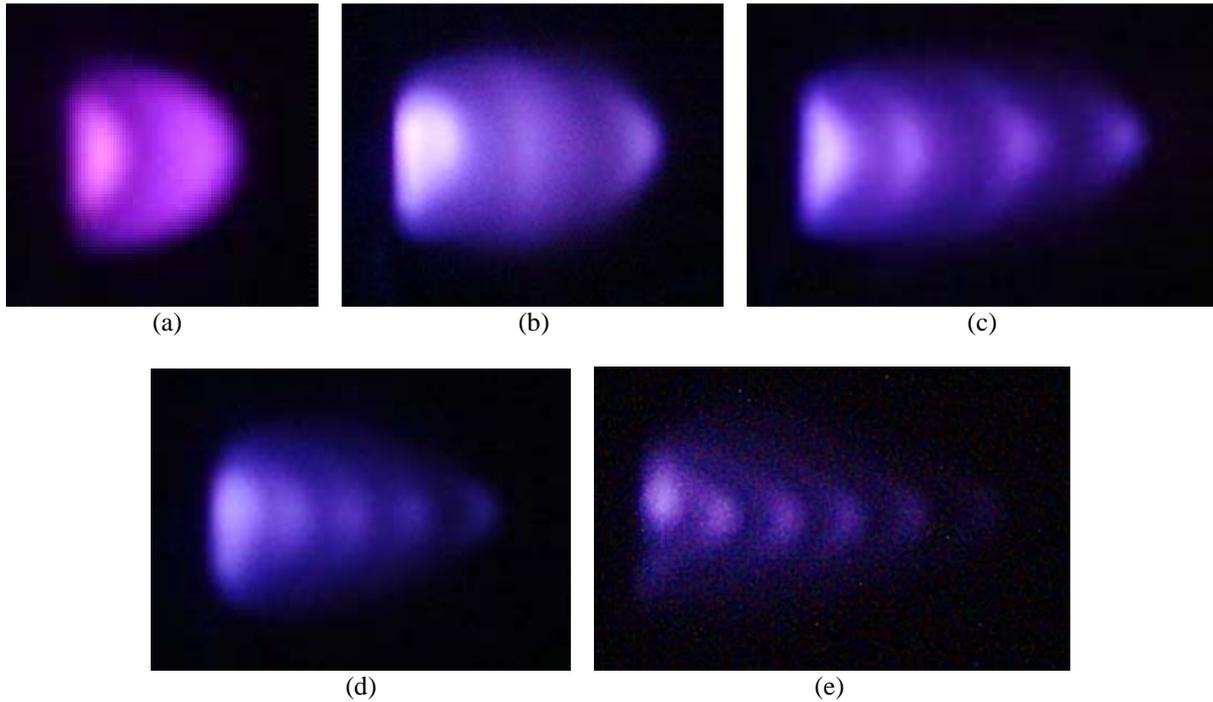
*Fig. 1: Photos of the multiple double layers in different stages (for different increasing values of the potential applied on the electrode)*
