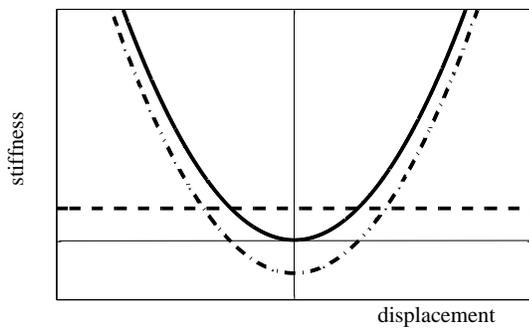
Figure 4. Qualitative plot of the stiffness as function of the displacement for the bistable plate (dash-dot), the mechanical spring (dashed) and the total stiffness of the isolator (solid)
