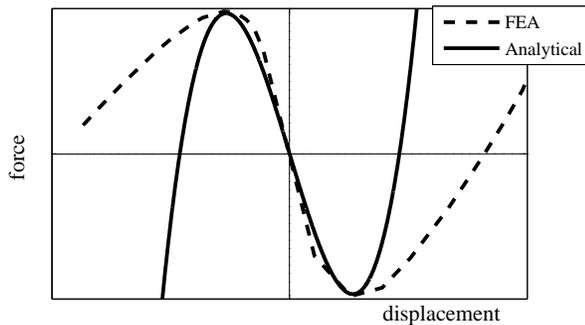
Figure 2. Load-deflection characteristic. The dashed line is obtained with finite element analysis (FEA), the solid line is the plot of the function  $f_p = -k_1 x + k_3 x^3$
