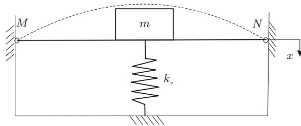
Figure 1. Schematic representation of a passive isolation system with a bistable plate and a mechanical spring. The dashed line indicate the plate in its initial shape. The addition of the mass  $m$  causes the plate to become approximately horizontal (solid line)
