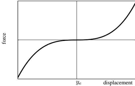
Figure 5. Load-deflection characteristic of the vibration isolator with a bistable plate and a mechanical spring. For oscillations about the static equilibrium position the stiffness is small and this results in a low natural frequency
