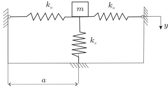
Figure 3. Mechanical SDOF model of the isolation system with a bistable plate, represented by two oblique springs of identical coefficient  $k_o$ , and a vertical mechanical spring  $k_v$
