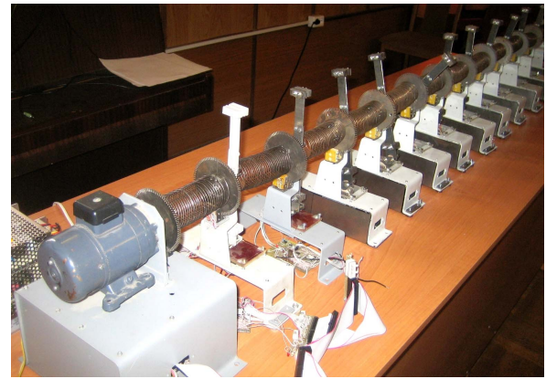
Figure 6. Photo of the chain pendulums and the motor.
