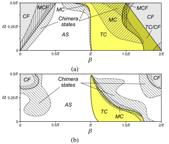
Figure 1. Diagrams of dynamical states of network with all-to-all connections (a) and random network with average node degree  $k = 10$  (b). The dynamical states of the network: (TC) - two-cluster state, (MC) - multi-cluster state, the states characterized by the formation of one (CF) or several (MCF) coherent groups with a fixed phase relationship between oscillators within the groups, (AC) - asynchronous state.
