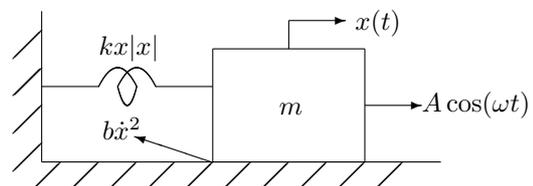
Figure 1. Scheme of nonlinear mass-spring model
