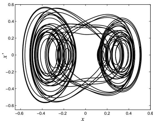
Figure 7. Phase portrait of the model corresponding to the chaotic behavior for  $\alpha = 8, \beta = 0.1, \gamma = 1$  and  $\omega = 0.1\pi$ .
