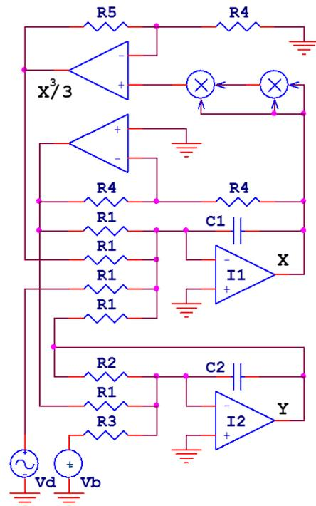
Figure 2. Electronic implementation of each FitzHugh-Nagumo system that composes a network.
