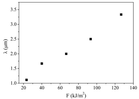
Figure 3. Dependence of the maximal cell size (in the centre of the crater) for aluminium sample on the pulse fluence.
