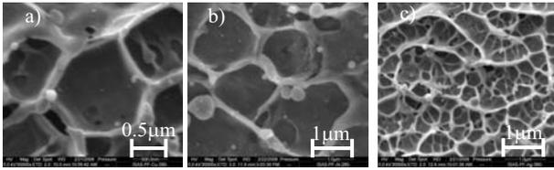
Figure 1. Typical laser crater. a) Cu,  $F=127 \text{ kJ/cm}^2$ ; b) Al,  $F=93 \text{ kJ/cm}^2$ ; c) Ag,  $F=127 \text{ kJ/cm}^2$ .
