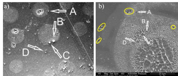
Figure 4. Copper sample a) before and b) after fs-laser ablation. Nanoparticles present on the surface before the ablation and corresponding Voronoi cells are marked with arrows. The cavities on the surface are marked in the both figures for the orientation. The figure size is approximately  $70 \mu\text{m}$
