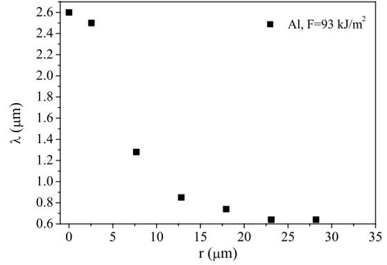
Figure 2. Dependence of the cell size along the crater radius.
