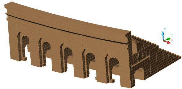
Figure 3. 3D model generated with AutoCAD software including 2670 blocks for five arches on the first floor.
