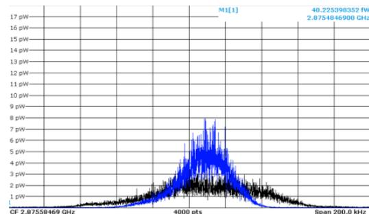
Figure 8. Experimental results of beam stochastic cooling of coasting <sup>12</sup>C<sup>6+</sup>. Schottky beam spectra: black – initial beam, blue – cooled beam. Coasting beam,  $I \sim 2e9$  ions,  $E \sim 2.5Gev/u$ ,  $\Delta p/p_{initial} \sim 0.15e-3$ ,  $\Delta p/p_{final} \sim 0.07e-3$ ,  $\tau_{cool} \sim 27$  sec
