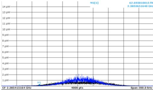
Figure 9. Experimental results of beam stochastic cooling of bunched  $^{12}\text{C}^{6+}$ . Schottky beam spectra: black – initial beam, blue – cooled beam. Right: bunched beam,  $I \sim 2e9$  ions,  $E \sim 2.5$  GeV/u,  $dp/p_{\text{initial}} \sim 0.2e-3$ ,  $dp/p_{\text{final}} \sim 0.13e-3$ ,  $\tau_{\text{cool}} \sim 64$  sec
