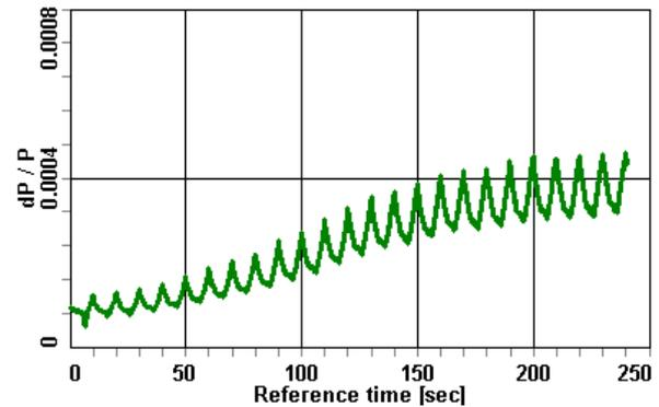
Figure 5. Accumulation with electron cooling and IBS: momentum spread. Ion energy E = 4.5 GeV/u.
