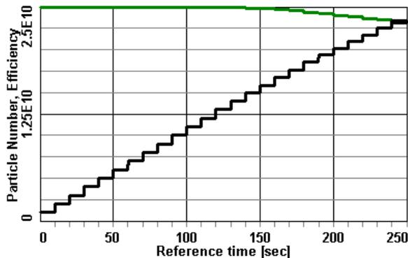
Figure 4. Accumulation with electron cooling and IBS: particle number (black) and accumulation efficiency (green). Ion energy E = 4.5 GeV/u.
