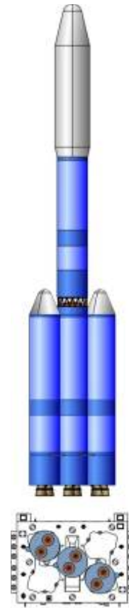
Fig. 5. Middle-class launch vehicle with increased lifting capacity with RD180 engines at first stage and RD0146 at second stage
