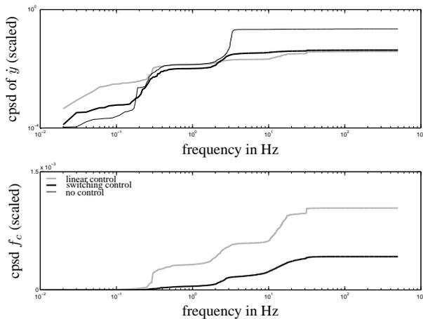
Figure 11. Cumulative power spectral density (cpsd) analysis of the payload velocity and control force in  $z$ -direction in case of no control, linear control, and switching control.
