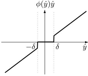
Figure 7. Switching characteristics of  $\phi(\dot{y})\dot{y}$ .
