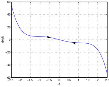
Figure 2. DF-PLL dynamical behavior of the equilibrium state for  $\alpha = -2$
