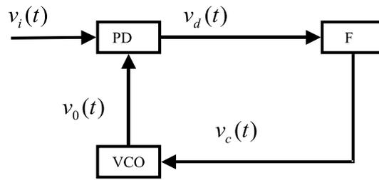
Figure 1. PLL block diagram
