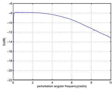
Figure 8. DF-PLL perturbation rejection
