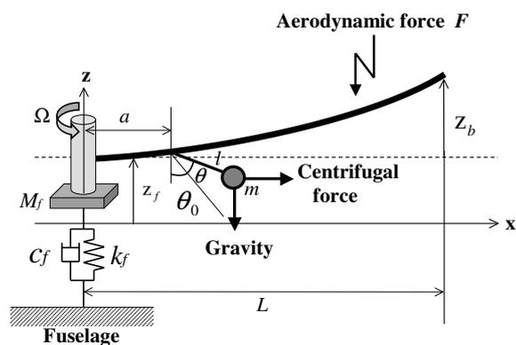
Figure 1. Model for a blade, a pendulum absorber and a rotor mount.
