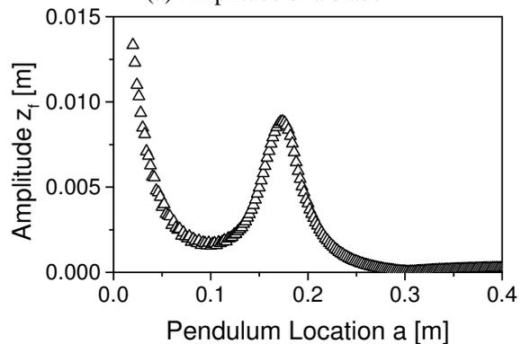
(b) Amplitude of a rotor mount
