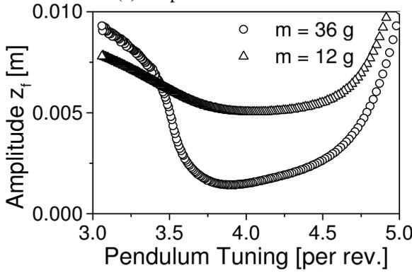
(b) Amplitude of a rotor mount
