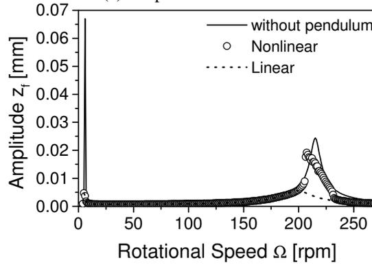
(b) Amplitude of a rotor mount
