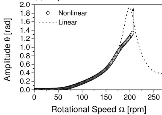
(c) Amplitude of a pendulum
