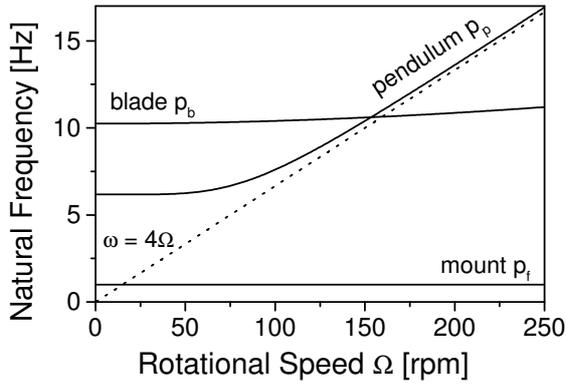
Figure 2. Natural frequencies of a blade, a pendulum absorber and a rotor mount
