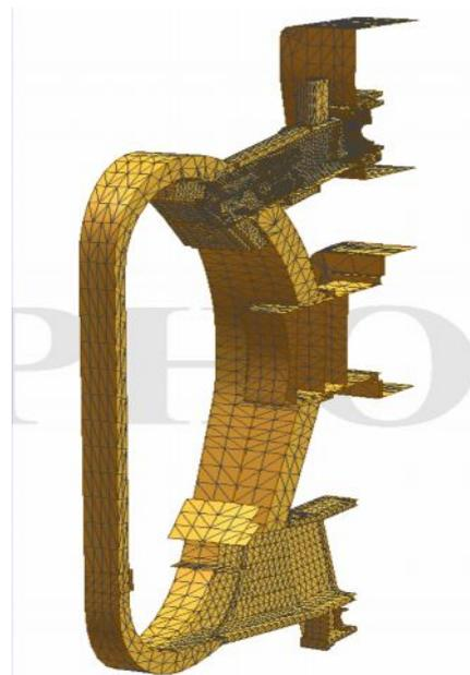
Figure 10. FE model of sector (1/36) with blanket modules #9-11. Inboard view
