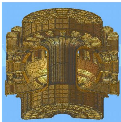
Figure 5. FE model of ITER VV and TS.
