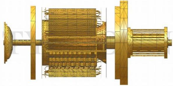
Figure 9. FE model of torus cryopump. The carrier tube of housing and carrier tubes of 80K radiation shield are not shown.
