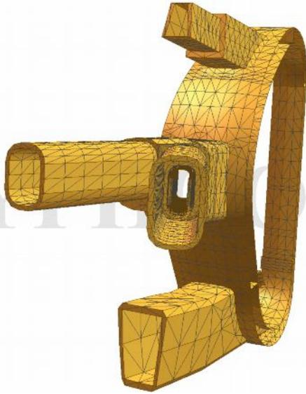
Figure 7. 20-degree sector of VV model. Heating neutral beam liner with cooling pipes is incorporated into heating/diagnostic neutral beam (H/DNB) equatorial port. Outboard view.
