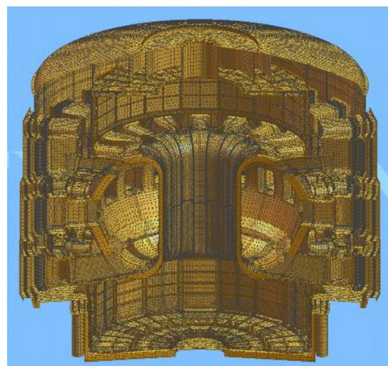
Figure 6. FE model of ITER VV+ cryostat +TS
