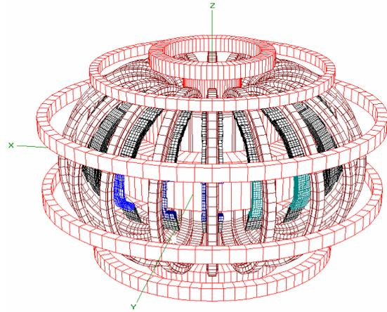
Figure 2. Model for ITER magnets and plasma
