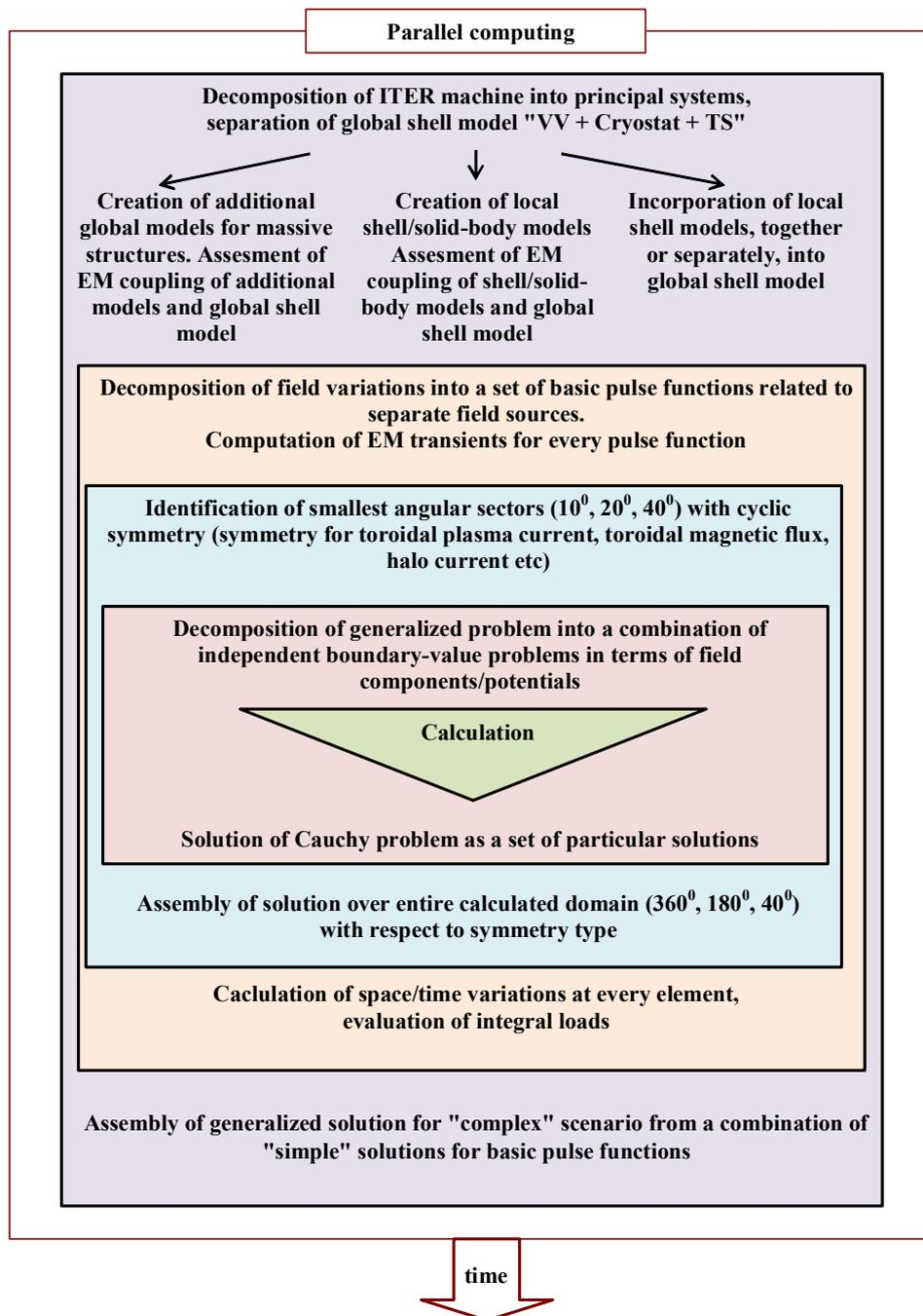
Figure 1. Algorithm for EM computations using parallelism
