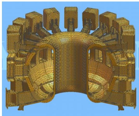
Figure 4. FE model of ITER VV
