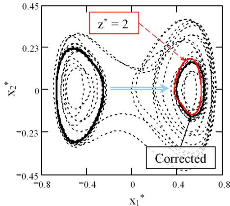
Figure 4. The solution of the problem (12): trajectories of the corrected system (18) in the phase space with  $a_{\min} = 0.05$ .
