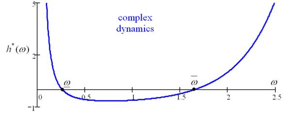
Figure 1. The regular and complex dynamics boundary at optimal static correction of the system (3) on parameter  $\beta$ .
