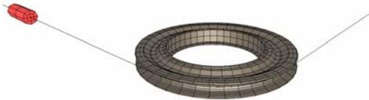
Fig. 6. Deck block and muffle
