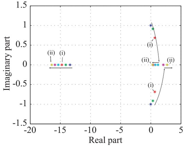
Figure 2. Root locus of  $A$  with  $\gamma=0.00272$ ,  $R=13.41$ , and  $P=0.3506$  under changing  $K_l$  from 0 to 50 ((i):  $K_l=20$ , (ii):  $K_l=50$ ).
