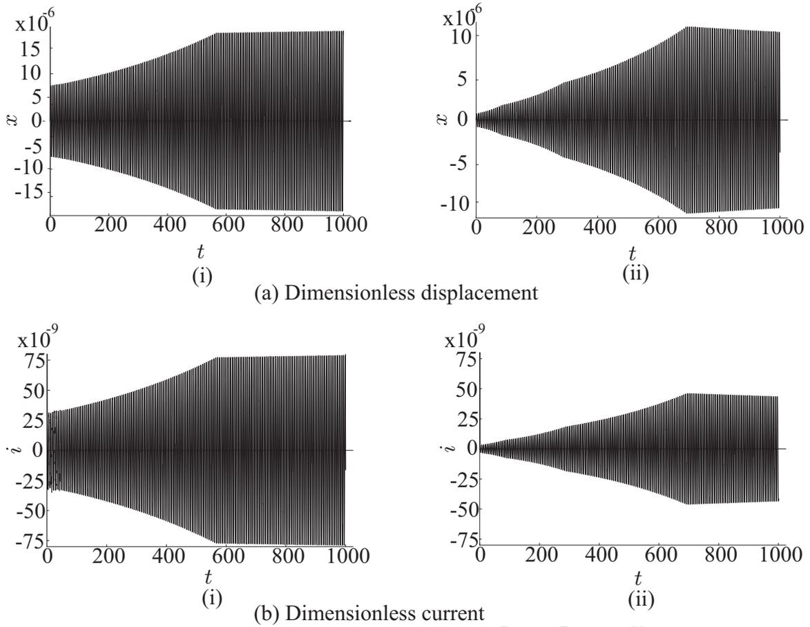
Figure 5. Time histories of dimensionless displacement and current with  $\gamma=0.00272$ ,  $R=13.41$ ,  $P=0.3506$ ,  $K_l=0.387$  and  $\epsilon=0.05$ . (i):  $\mu=10$ , (ii):  $\mu=1000$ .
