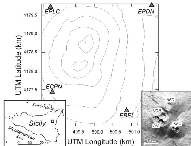
Figure 1. Map of the summit area of Mt. Etna with the location of the four infrasonic sensors (triangles), composing the permanent infrasound network. The digital elevation model in the lower right corner shows the distribution of the four summit craters (VOR=Voragine, BN=Bocca Nuova, SEC=South-East Crater, NEC=North-East Crater).
