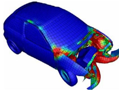
Figure 9. Deformed vehicle after stop, the plastic strain intensity.
