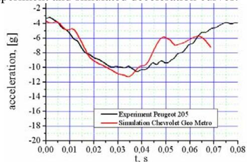
Figure 7. Deceleration curve obtained at FEM at 100km/h impact speed in comparison with experiment
