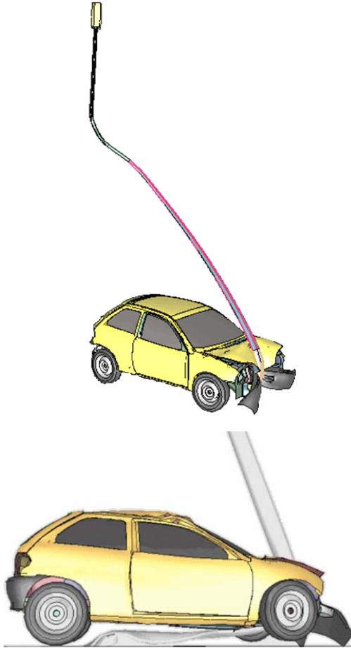
Figure 5. Column impact and sliding under vehicle
