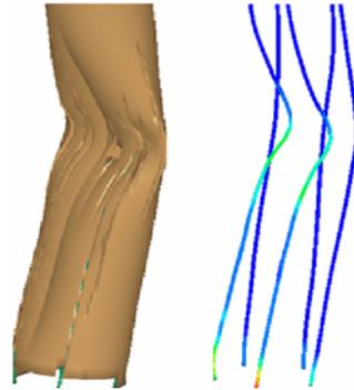
Figure 6. Progressive damage at column laminate and equivalent plastic strain in reinforcing bars
