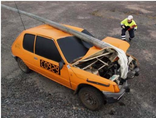
Figure 2. Deformed column and vehicle after impact of 100 km/h. Impact tests performed by Helsinki University of Technology, Laboratory of Highway Engineering
