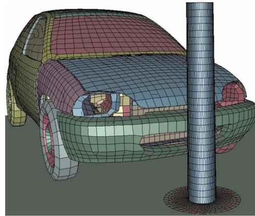
Figure 3. Three-dimensional finite element model
