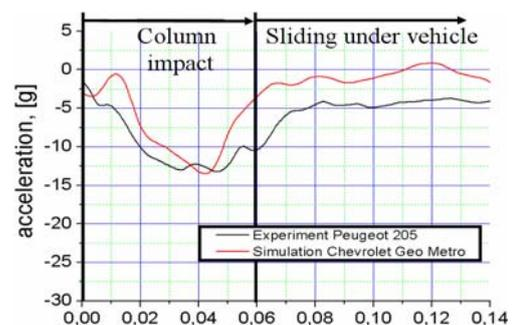
Figure 4. Deceleration curve obtained at FEM at 100km/h impact speed in comparison with experiment
