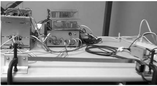
Fig. 1. The experimental system actuated by a piezoelectric actuator
