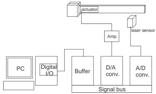
Fig. 2. Schema of the experimental system
