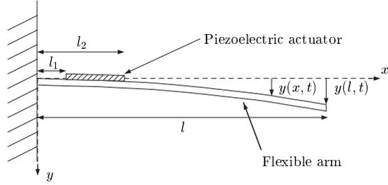
Fig. 3. Schema of the flexible arm with the piezoelectric actuator
