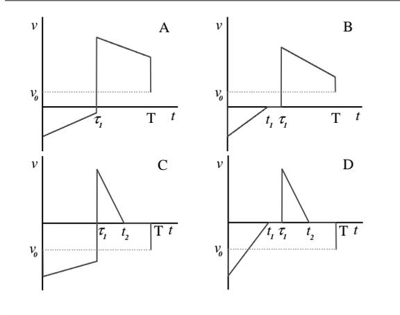
Fig. 4. Modes of motion in the presence of dry friction
