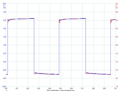
Figure 10. Experimental result of the system with the synchronization control law activated (blue-line is the master's output, and red-line is the slave's output).
