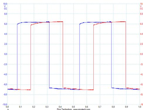
Figure 9. Experimental result of the system without the synchronization control law (blue-line is the master's output, and red-line is the slave's output).
