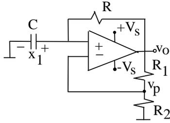
Figure 1. Basic astable multivibrator circuit.
