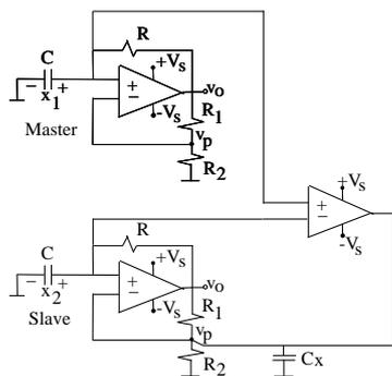
Figure 6. Electronic circuit.
