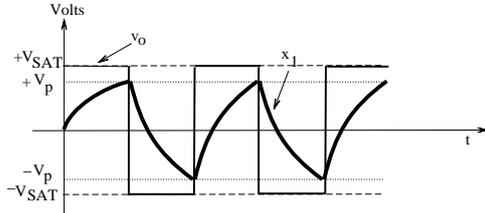
Figure 2. Waveforms for the free-running multivibrator ( $\pm V_{SAT}$  are the saturating voltages).
